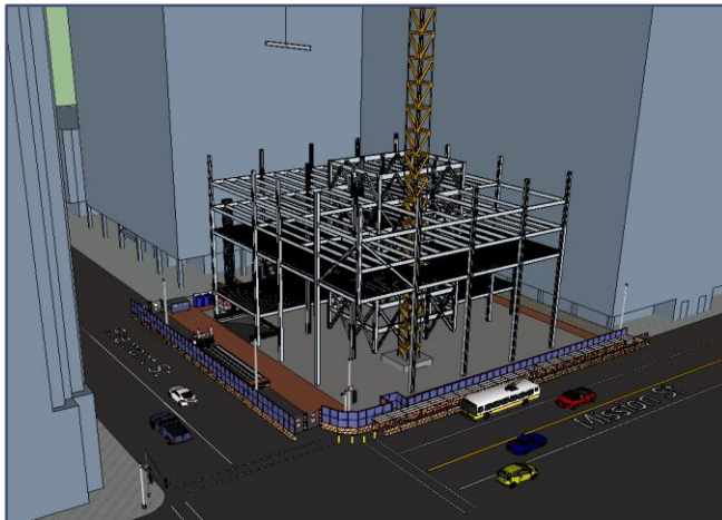
Figure I: Steel Erection Phase
